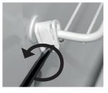
2. Tilt the shelf to one side at an angle while pulling forward.
