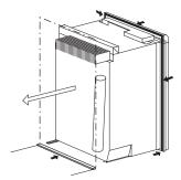
**Note!** Be careful not to damage the sealing strip when the refrigerator is put in place.
