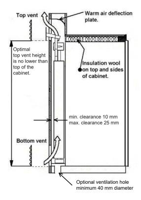
**Notice:** If the design of the vehicle does not allow you to install the top exhaust vent directly above the condenser of the refrigerator (what Dometic recommends):
