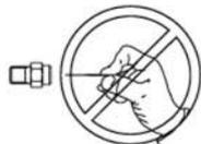
10. Before removing burner jet, clean burner area of soot and scale that fell out of flue tube.
