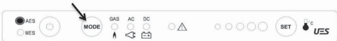
Note AES function should only be used when a suitable D+ connection is made to the tow vehicle. See full instructions for details.
