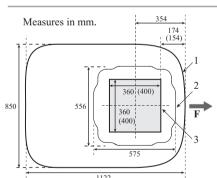
required on the ceiling for the plenum installation. Measure from the reference position of the 360×360mm (400×400mm) square hole.Remember to add 100mm clearance around roof top unit perimeter.
