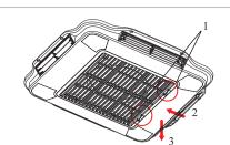
• Remove the air filter from the plenum by pushing both tabs inwards and then downwards.
